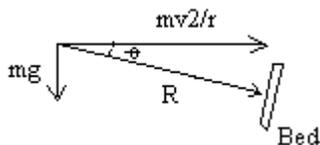
Here, as r goes on decreasing,  $\theta$  also decreases. So, bed of sliding goes on inclining to horizontal. (As it is perpendicular to R always.)
