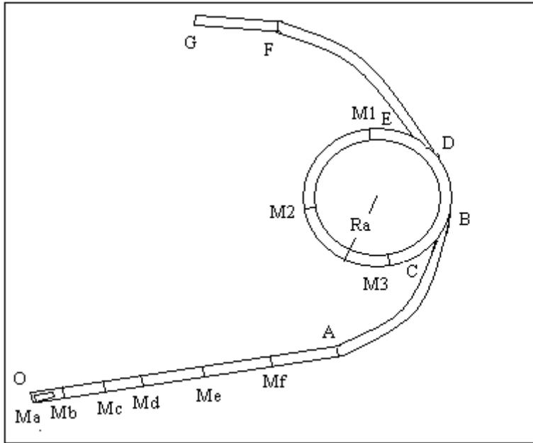
In between A & B radius of curvature goes on decreasing & by similar rate bed goes on inclining to horizontal. (As weight of space bullet remains same but centripetal force goes on increasing. Hence resultant of both becomes more and more horizontal.)
