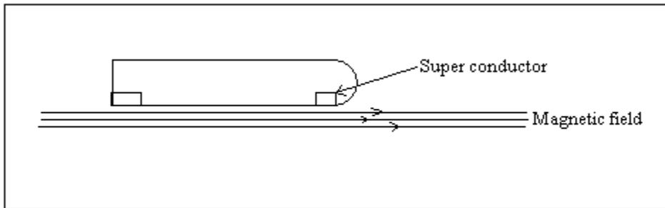
By law of nature, whenever we keep super conductor in magnetic field opposite field is formed by superconductor, pushes the super conductor in direction away from field.
